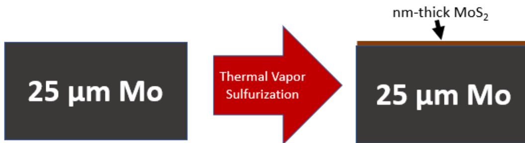
Figure 4-6 Modified TVS growth to use molybdenum foil as a growth substrate to yield a thin MoS 2 surface layer, with a large Mo layer remaining underneath.
