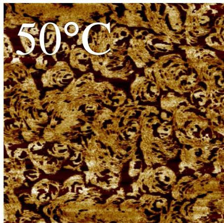
**Figure A8.** Morphology evolution as a function of temperature showing the melting transition starting at 45°C in 45 kDa PCL/SIS vector 4293A blend film exhibiting the nano-rose morphology.
