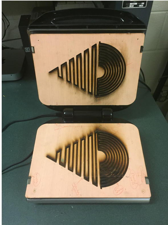
Figure 24: 1 st iteration plywood plating snapped in to press construct.
