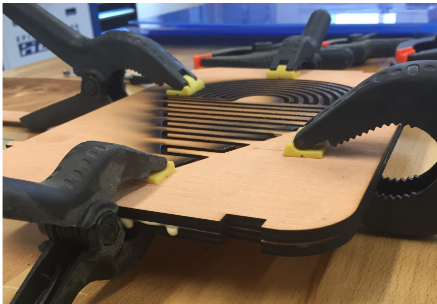
Figure 23: Fabrication of 1/2" thick plywood plate constructs.
