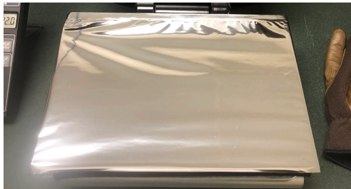
Figure 32: Sheet placed in tension on scrap piece of 6061 Aluminum for sealing process.
