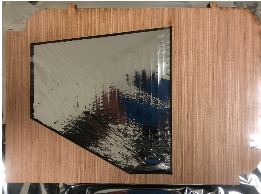
Figure 38: Sample preparation template made from Plywood with distinct areas for ASTM D642 Burst Testing.
