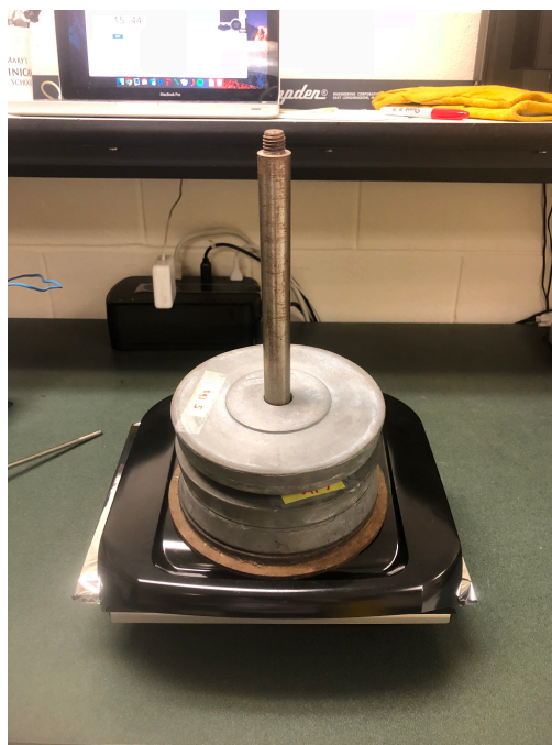
Figure 31: 20lb weight stack added to top of press construct for sealing. Applied for each dwell time in sample preparation.
