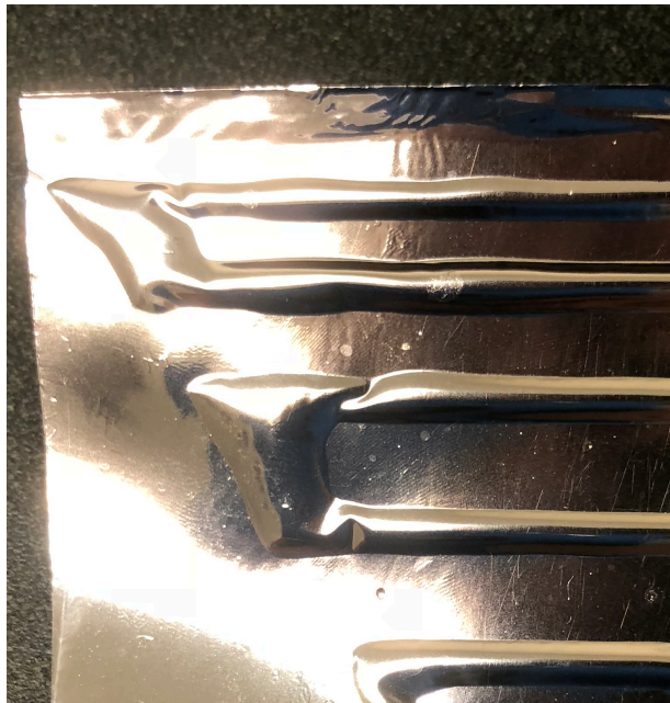
Figure 67: Presence of fluid pockets at >90 degree corners.
