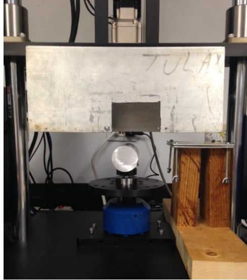
Figure 23: Beam-with-Overhang test apparatus
