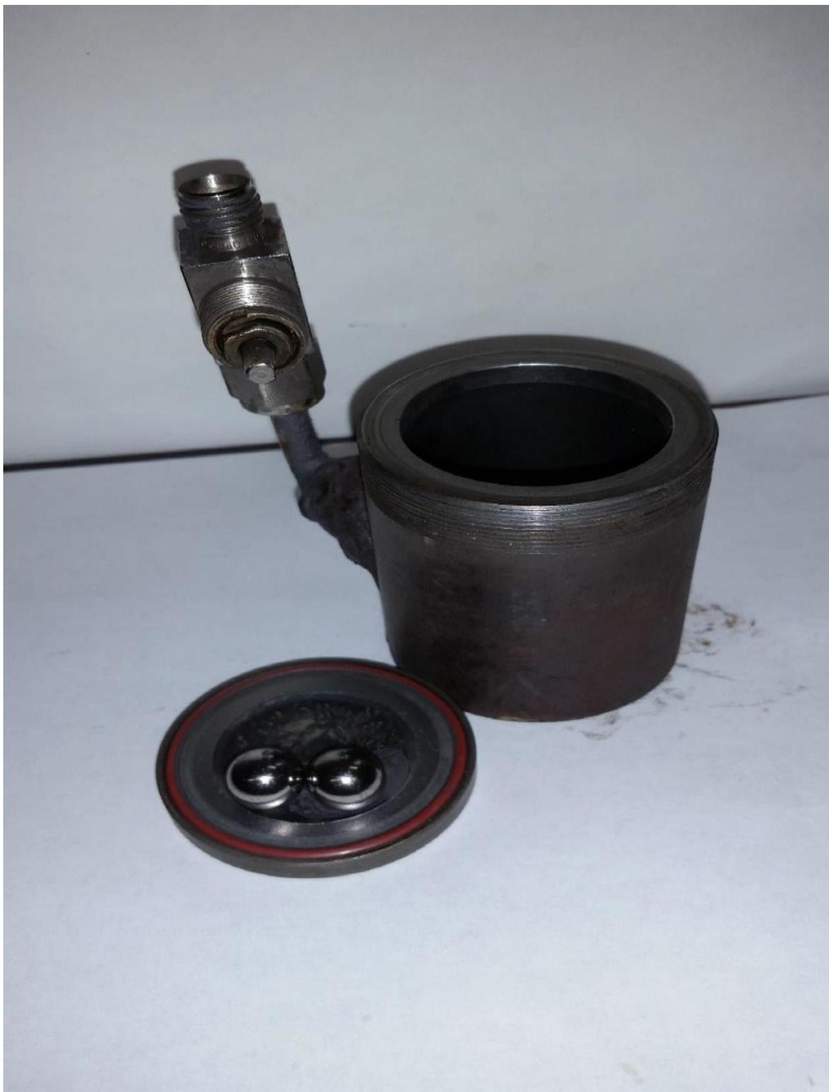
Figure 5.1. Stainless steel milling vial with adapted gas sidearm.
