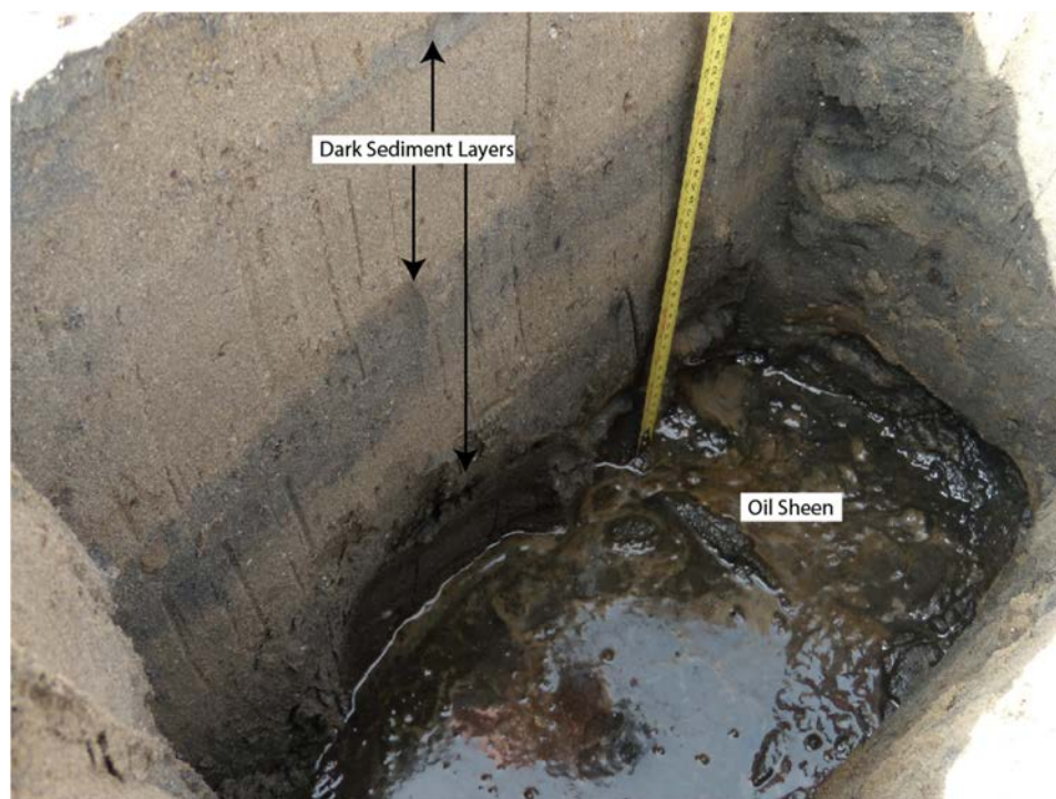
Figure 2.2. Sediment samples from Grand Isle were collected by digging trenches and sampling from dark bands and the trench bottom. An oil sheen was often observed on the water at the trench bottom, as well as an odor similar to that of oil. Image courtesy of B. Rosenheim.
