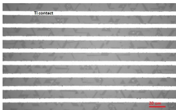
Figure C.2: CVD synthesized \text{MoS}_2 flakes on C-plane sapphire substrate with unidirectional orientation. One edge of the flakes is parallel to the phototransistor's Ti contact fingers.
