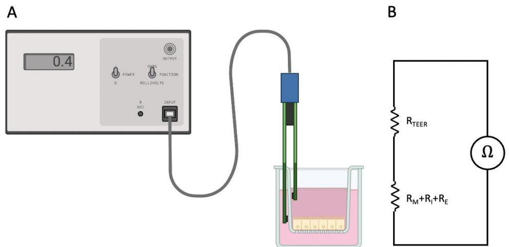
Figure 25: Schematic for the TEER measurement system.
