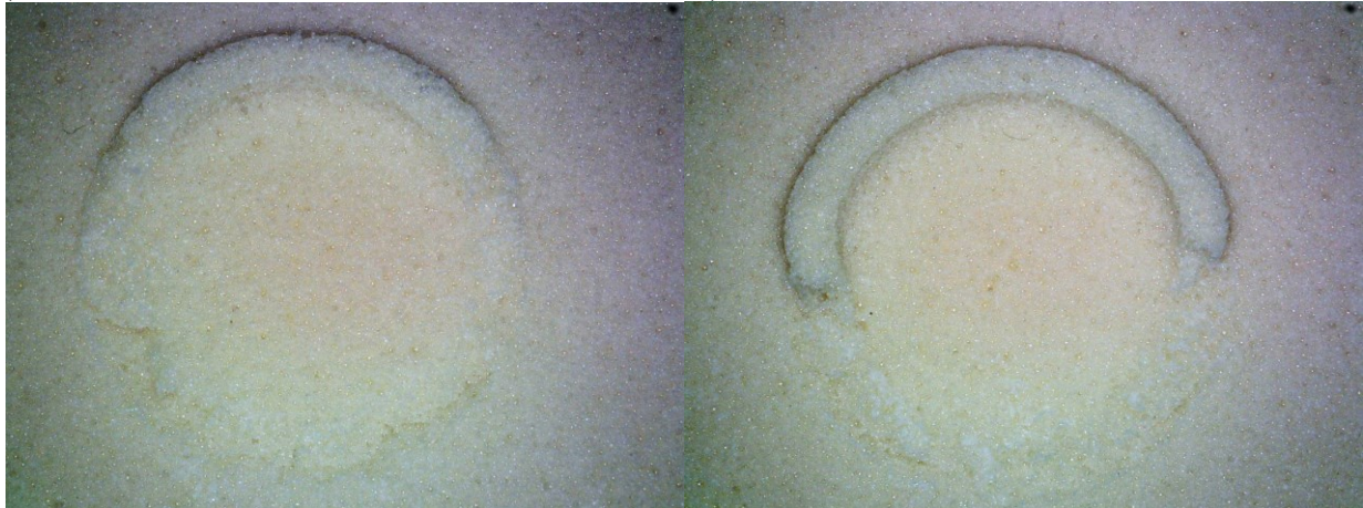
Image 29 Microscope images for sharp edge with through-growth: Trial 1 (a) angled block and (b) straight block
