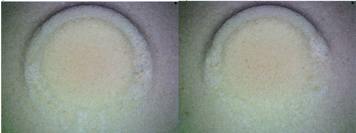
Image 21 Microscope images for curved edge with through-growth: trial 3 (a) angled block and (b) straight block
