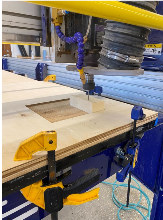
Image 6 ShopBot CNC machine used to cut foam blocks
