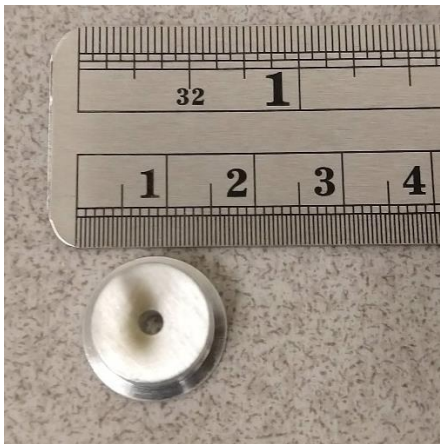
Figure 3-9 Misaligned laser aperture removed
