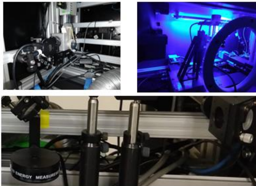
Figure 3-3 Laser energy meters (clockwise from top left): in line, work surface, in situ
