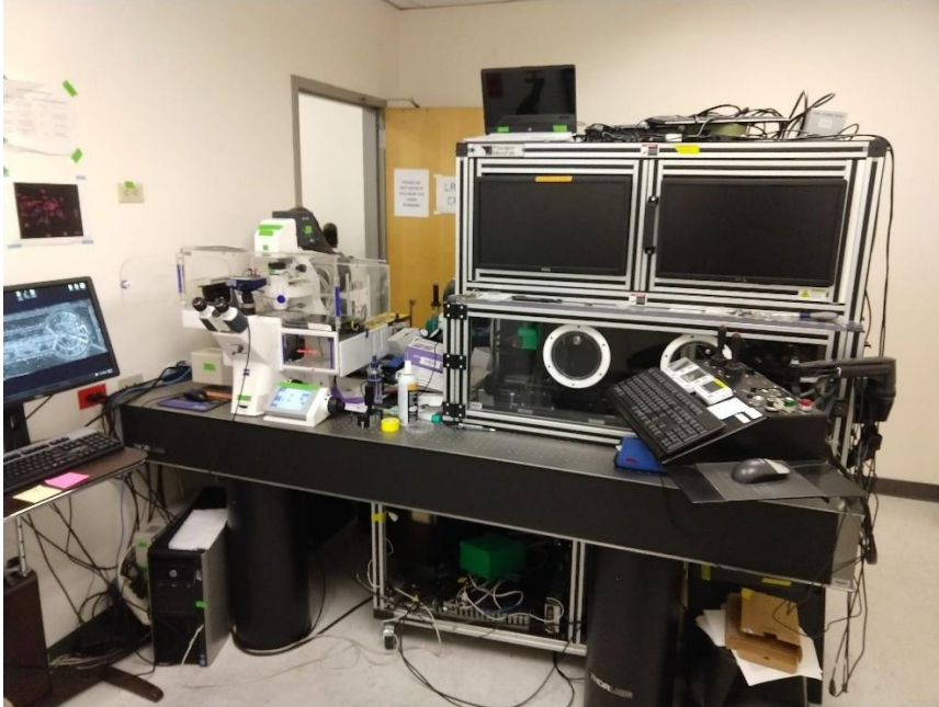
Figure 3-23 Convenient placement of the two additional computers required to control the Z-stages and energy meters (laptop) and the variable aperture (microscope computer)
