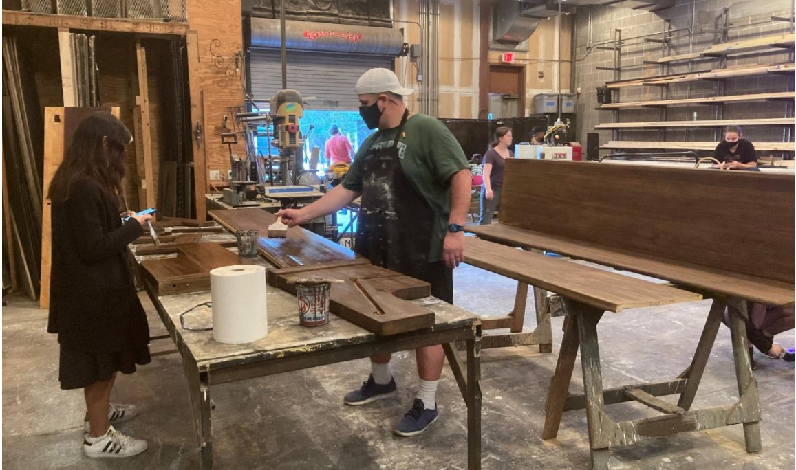
Figure 75: After sanding, each part of the pews is stained in a darker finish. 2021, Tulane University.
