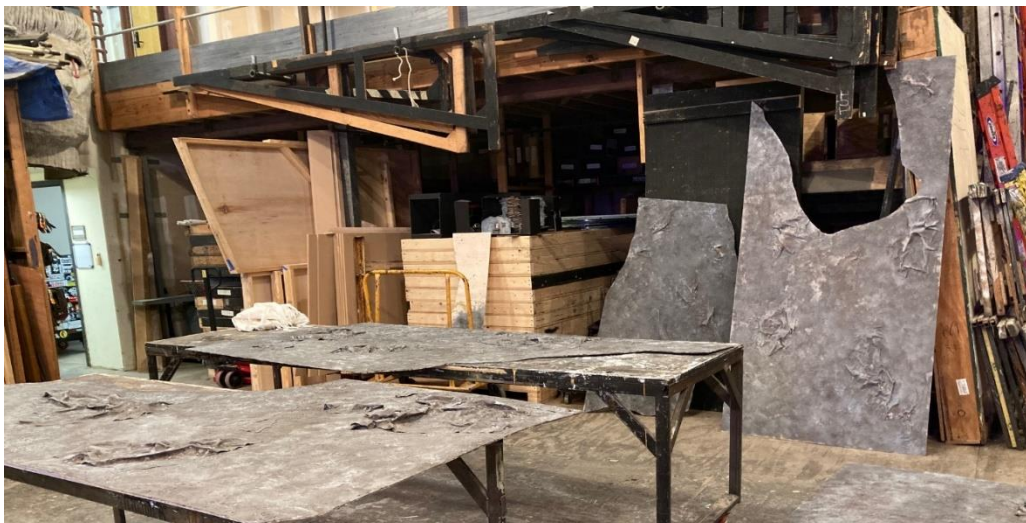
Figure 63: Sections of the upstage wall plaster drying after being sponged with paint. 2021, Tulane University.
