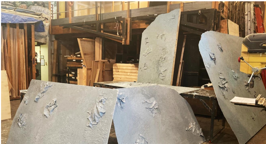
Figure 62: The downstage wall flats after the basecoat of plaster and paper. 2021, Tulane University.
