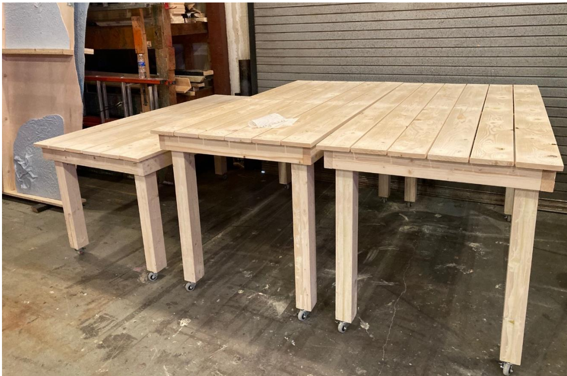
Figure 61: The worktables after construction and puttying all holes. 2021, Tulane University.
