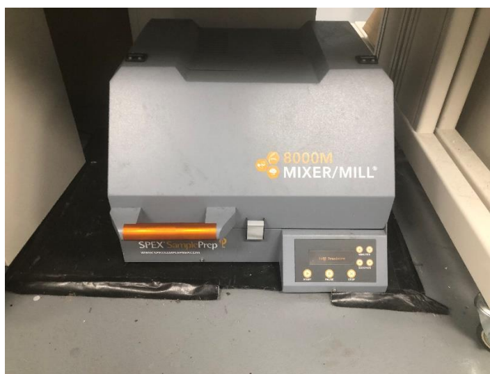
Figure 3.5: The SPEX mill used to prepare the carbonized material
