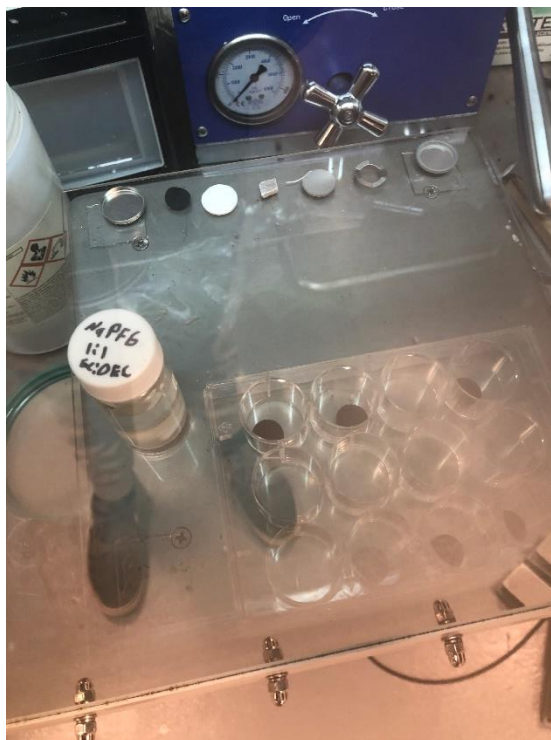
Figure 3.7: (From Left to Right) The positive battery lid, an electrode, the glass fiber separator, a piece of raw sodium, the stainless-steel current collector, a washer spring, and the negative terminal of the coin cell. Also pictured is a bottle of the NaFP 6 electrolyte.
