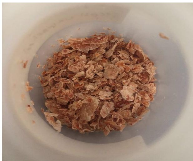
Figure 4.4: (A) Deproteinized chitin dominant crawfish after being soaked in NaOH. (B) EDS produced table showing the elemental weight and atomic percents of the NaOH soaked crawfish after washing.
