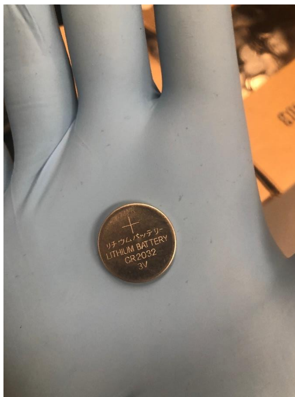
Figure 3.9: An assembled CR2032 coin cell
