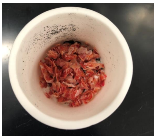
Figure 4.5: (A) Deacetylated chitosan dominant crawfish shells after being refluxed in KOH. (B) EDS produced table showing the elemental weight and atomic percents of the KOH refluxed crawfish.
