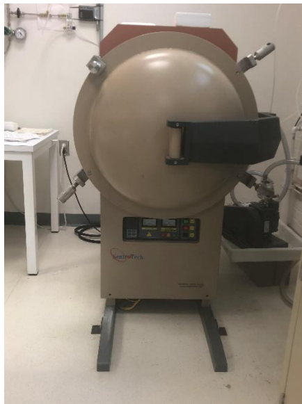
Figure 3.3: The vacuum furnace for the carbonization step
