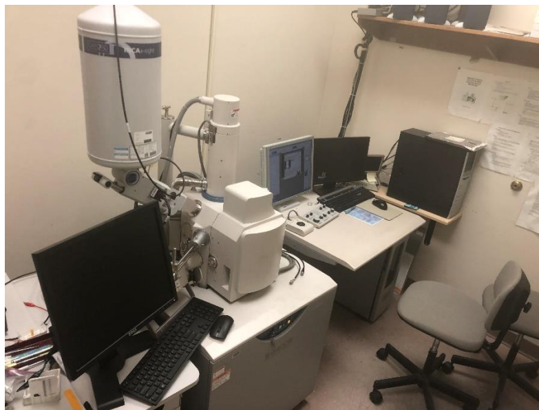
Figure 3.4: Hitachi S-3400 SEM used for EDS measurements
