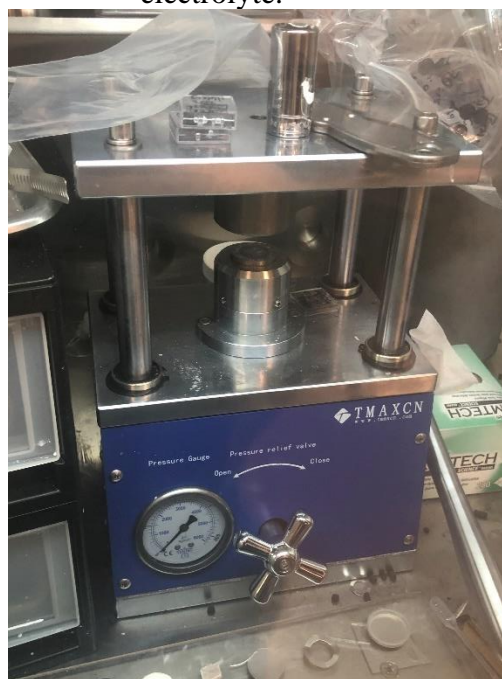
Figure 3.8: The cell press used to crimp the coin cells
