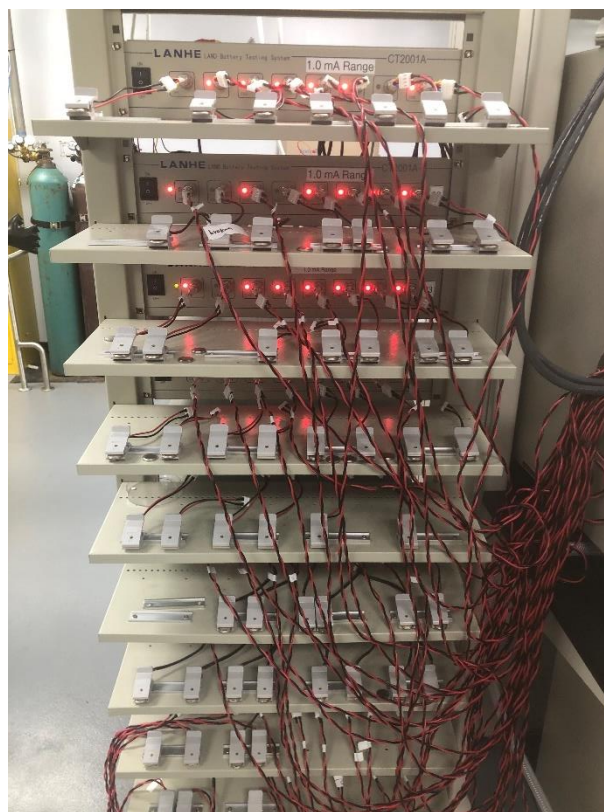
Figure 3.10: The LANHE cyclor channels with connections running to the environmental chamber adjacent
