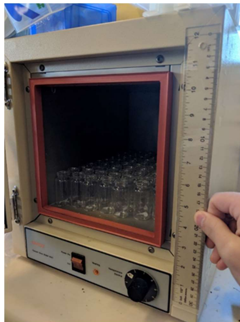
Figure 2.2: Drug loading set-up of p(HEMA) disks. Individual p(HEMA) disks, each in its own 20 mL vial, arranged in a single layer. This small portable vacuum oven can hold 70 vials in one layer, or the vials could be stacked to load up to 140 disks at one time.
