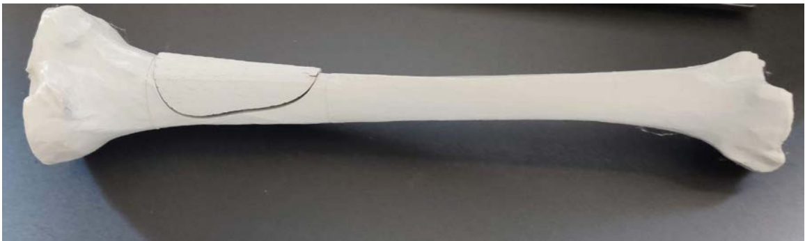
Figure 4.10.2 – Physical representation of lattice implant fit into the resected tibia
