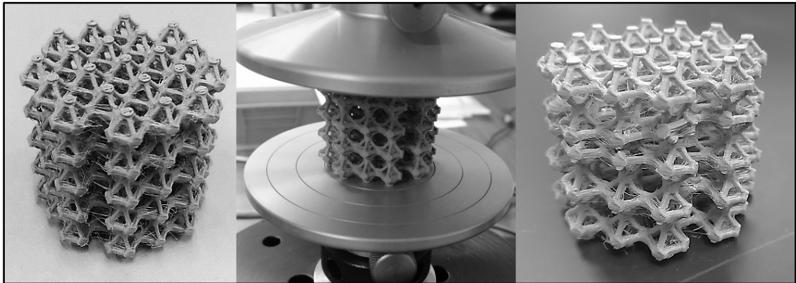
Figure 3.4.1 – (Left) 3D printed cylindrical lattice specimen, (Middle) Printed Lattice Experimental Setup, (Right) Visible fracture and deformation on printed lattice after 25% strain applied.
