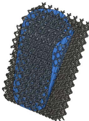
Figure 3.6.3 – Using incision surface to split the lattice body to contour to the estimation of the bone's outer body.
