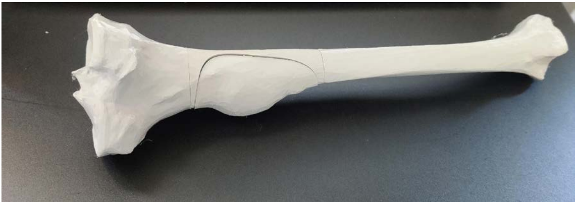
Figure 3.9.2 – Printed tibial specimen with detachable osteosarcoma.
