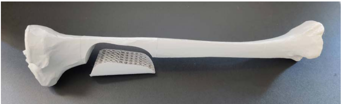
Figure 4.10.1 – Physical representation of lattice implant overlaid by the resected tibia
