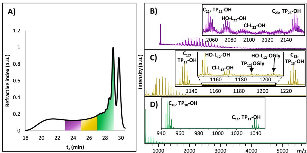
**Figure 4.6.** Poly(ECH) was fractionated by SEC (A), and the corresponding MALDI-ToF mass spectra of each SEC fraction is shown (B, C, and D). The spectra were acquired in reflector mode, and all signals represent the sodiated adducts.
