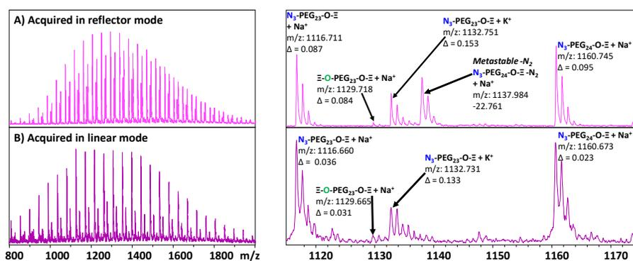
**Figure 6.2.** MALDI-TOF MS data of the  $\alpha$ -azido- $\omega$ -propargyl-PEG
