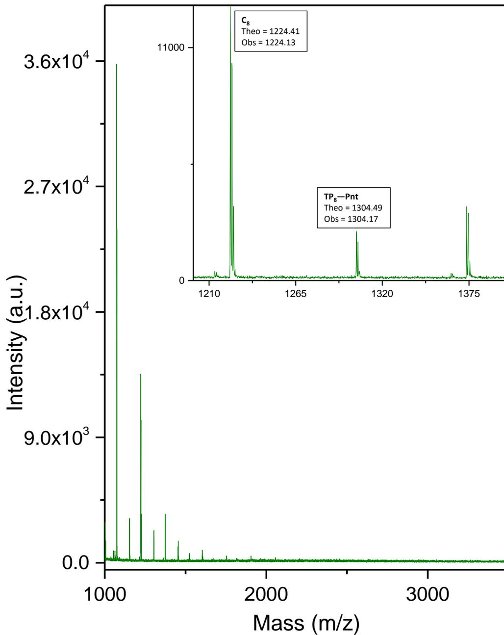
**Figure B8.** MALDI-ToF mass spectrum of pent-4-ynoated poly(GPE)<sub>11K</sub> sample was taken in positive reflector mode, and all labeled signals represent the sodiated adducts.
