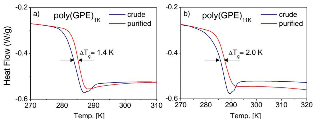
**Figure 3.9.** DSC data for crude and purified cyclic poly(GPE) samples. a) poly(GPE)<sub>1K</sub> and b) poly(GPE)<sub>11K</sub>.
