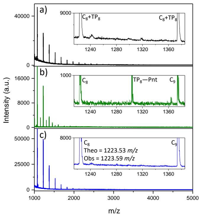
**Figure 3.4.** MALDI-TOF mass spectra of (a) crude poly(GPE)<sub>11K</sub> sample, (b) poly(GPE)<sub>11K</sub> product after esterification with 4-pentynoic acid, and (c) “click-scavenged” poly(GPE)<sub>11K</sub>, with expanded spectra from  $m/z = 1215$  to  $1385$   $m/z$  in each inset. The spectra were taken in positive reflector mode, and all labeled peaks represent the sodiated adducts.
