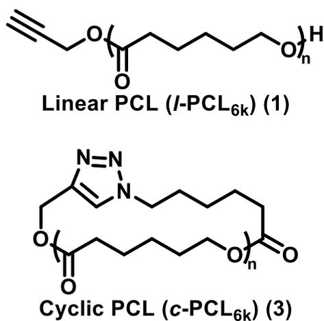
**Figure 5.1.** Structures of *l*-PCL<sub>6k</sub> and *c*-PCL<sub>6k</sub>. The numbers (1) and (3) correspond to the synthetic identification of these polymers in the “Synthetic Protocols” section of the Supporting Information.
