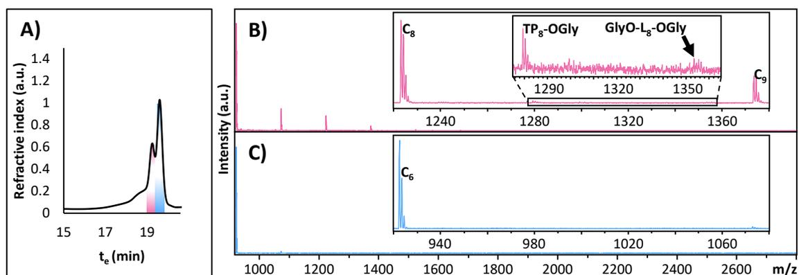
**Figure C1.** Poly(PGE) was purified via “click-scavenging” and fractionated by SEC (A), and the corresponding MALDI-ToF mass spectra of each SEC fraction is shown (B and C). Identification of signals is based on the end group functionalization performed in a previous study.<sup>3</sup> The spectra were acquired in reflector mode, and all signals represent the sodiated adducts.
