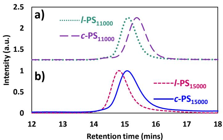
**Figure 2.6.** GPC chromatograms of (a) *l*- and *c*-PS<sub>10k</sub> and (b) *l*- and *c*-PS<sub>14k</sub>. Both sets of chromatograms illustrate a longer retention time for the cyclic analog due to reduced hydrodynamic volume.
