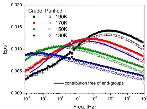
**Figure 3.11.** Dielectric relaxation for crude and purified poly(GPE)<sub>1K</sub> well-below  $T_g$ . Solid line shows the contribution to local dynamics of side groups (end groups are excluded) at 170 K, as previously obtained from linear poly(GPE) samples in reference.<sup>23</sup>
