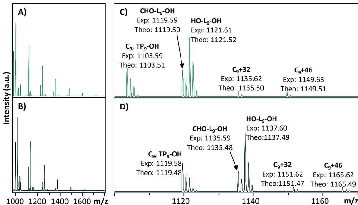
**Figure C9.** MALDI-ToF mass spectra of the low molecular poly(SO) fraction collected using Na<sup>+</sup> as a cation (A, C) and K<sup>+</sup> as a cation (B, D). All signals shift by a nominal mass of + 16 m/z from the Na<sup>+</sup> (C) to K<sup>+</sup> (D) spectra, confirming the assignment of signals is based on the proposed structure plus the added cation source.
