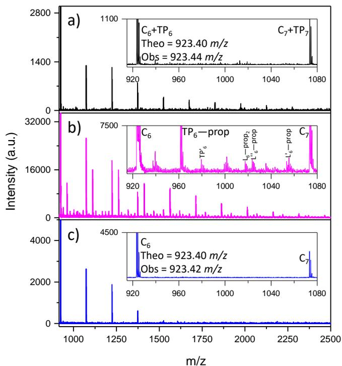
**Figure 3.3.** MALDI-TOF mass spectra of (a) crude poly(GPE)<sub>1K</sub> sample, (b) propargylated poly(GPE)<sub>1K</sub>, and (c) "click-scavenged" poly(GPE)<sub>1K</sub>, with expanded spectra from  $m/z = 915$  to  $1080$  in each inset. The spectra were taken in positive reflector mode, and all labeled signals represent the sodiated adducts.
