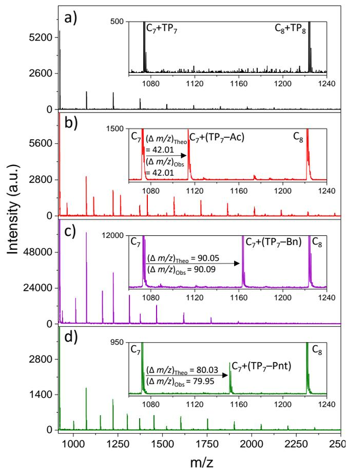
**Figure 3.2.** MALDI-TOF mass spectra of (a) crude poly(GPE)<sub>1K</sub> sample, (b) acetylated poly(GPE)<sub>1K</sub>, (c) benzylated poly(GPE)<sub>1K</sub>, and (d) the pentynoate ester of poly(GPE)<sub>1K</sub>, respectively, with expanded spectra from  $m/z = 1060$  to  $1240$  in each inset. The spectra were taken in positive reflector mode, and all labeled signals represent the sodiated adducts.
