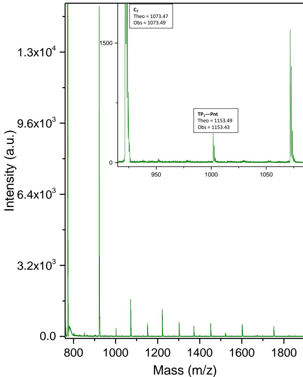
**Figure B6.** MALDI-ToF mass spectrum of pent-4-ynoated poly(GPE)<sub>1K</sub> sample was taken in positive reflector mode, and all labeled signals represent the sodiated adducts.
