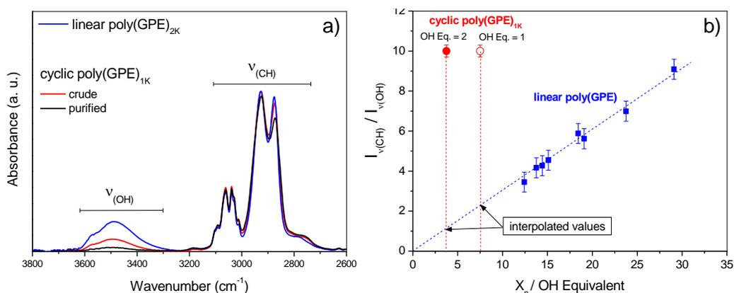
**Figure 3.6.** a) FTIR spectra of crude and purified cyclic poly(GPE)<sub>1K</sub> sample obtained by ZREP and a linear poly(GPE) standard ( $M_n = 2.2$  kg/mol) synthesized by Endo's method.<sup>20</sup> b) Calibration curve obtained from linear poly(GPE) standards and FTIR data obtained for crude cyclic poly(GPE)<sub>1K</sub> considering OH Equivalent = 1 and 2.
