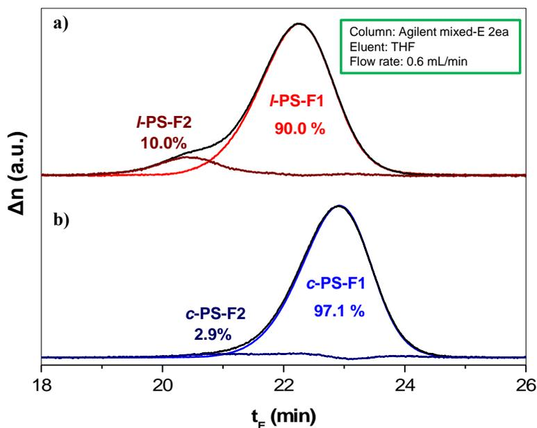
**Figure A6.** Representative SEC chromatograms of HPLC fractions 30 days after azidation and cyclization for a) *l*-PS<sub>2800</sub> and b) *c*-PS<sub>2800</sub>. Fraction 1 corresponds to the isolated unimer fraction, while fraction 2 corresponds to the dimer fraction.
