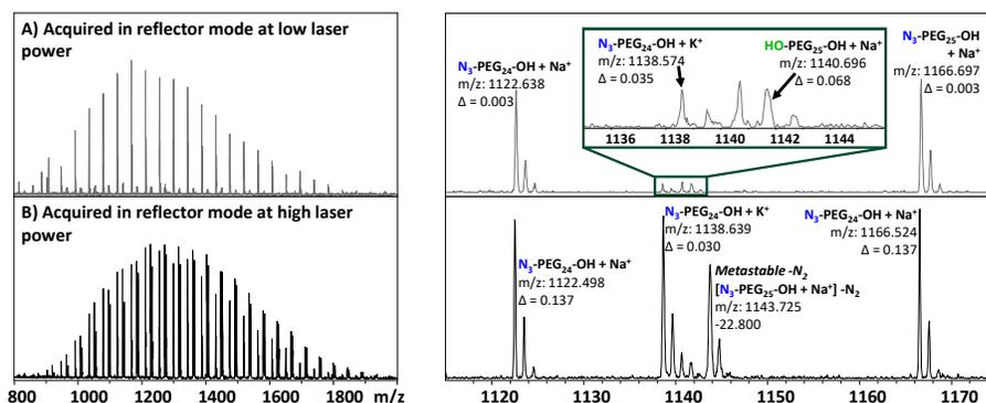
**Figure 6.1.** MALDI-TOF MS data of the  $\alpha$ -azido- $\omega$ -hydroxy-PEG linear precursor
