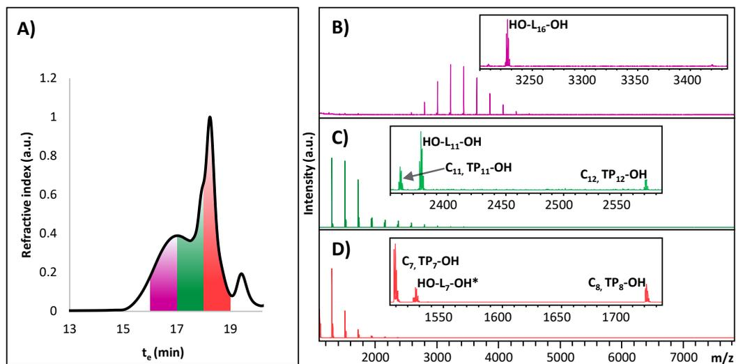
**Figure 4.5.** Poly(ETD) was fractionated by SEC (A), and the corresponding MALDI-ToF mass spectra of each SEC fraction is shown (B, C, and D). Identification of signals is based on the end group functionalization (**Figure C6**). Please note that the asterisk (\*) adjacent to HO-L<sub>7</sub>-OH is a result of two overlaying signals, which are further depicted in **Figure C5**. The spectra were acquired in reflector mode, and all signals represent the sodiated adducts.
