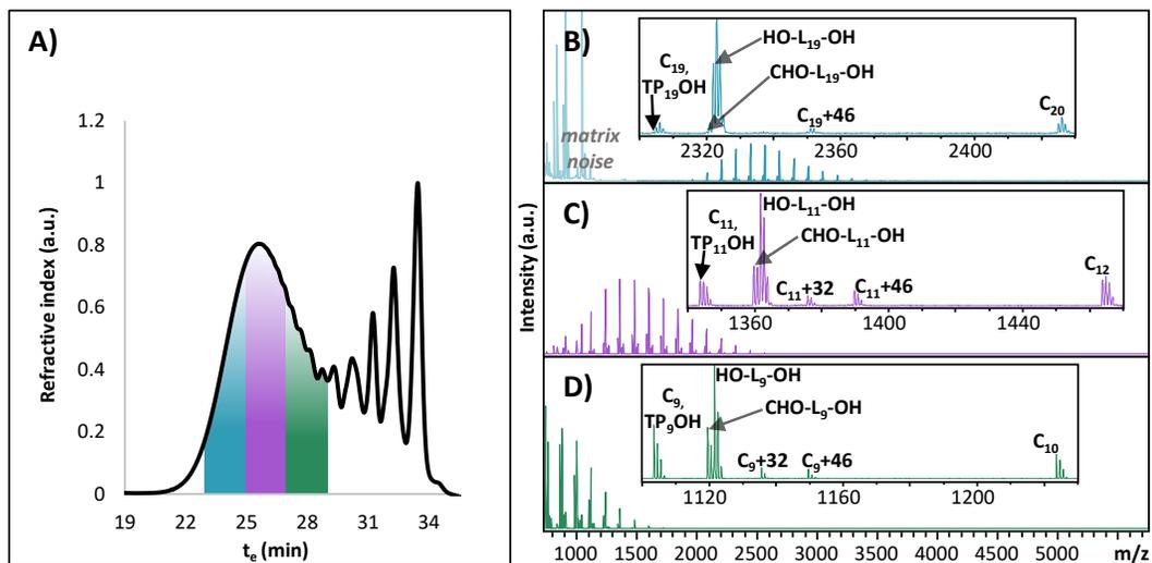
**Figure 4.7.** Poly(SO) was fractionated by SEC (A), and the corresponding MALDI-ToF mass spectra of each SEC fraction is shown (B, C, and D). Identification of signals is based on the end group functionalization (**Figure C7**). The spectra were acquired in reflector mode, and all signals represent the sodiated adducts.
