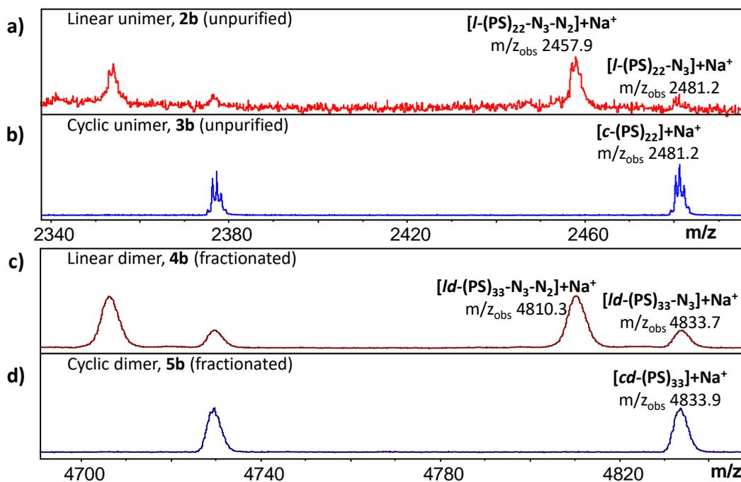
**Figure A3.** MALDI-TOF mass spectra in reflector mode of a) *l*-PS<sub>2800</sub>, b) *c*-PS<sub>2800</sub>, c) *ld*-PS<sub>2800</sub>, d) *cd*-PS<sub>2800</sub> confirming the loss of the predominant metastable azide signal upon CuAAC cyclization to form the triazole linkage in the cyclic products.
