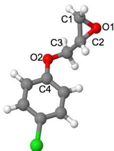
**Figure C2.** Atomic labeling within the X-PGE monomers, where X = H, Cl, NH<sub>2</sub>, and CN.
