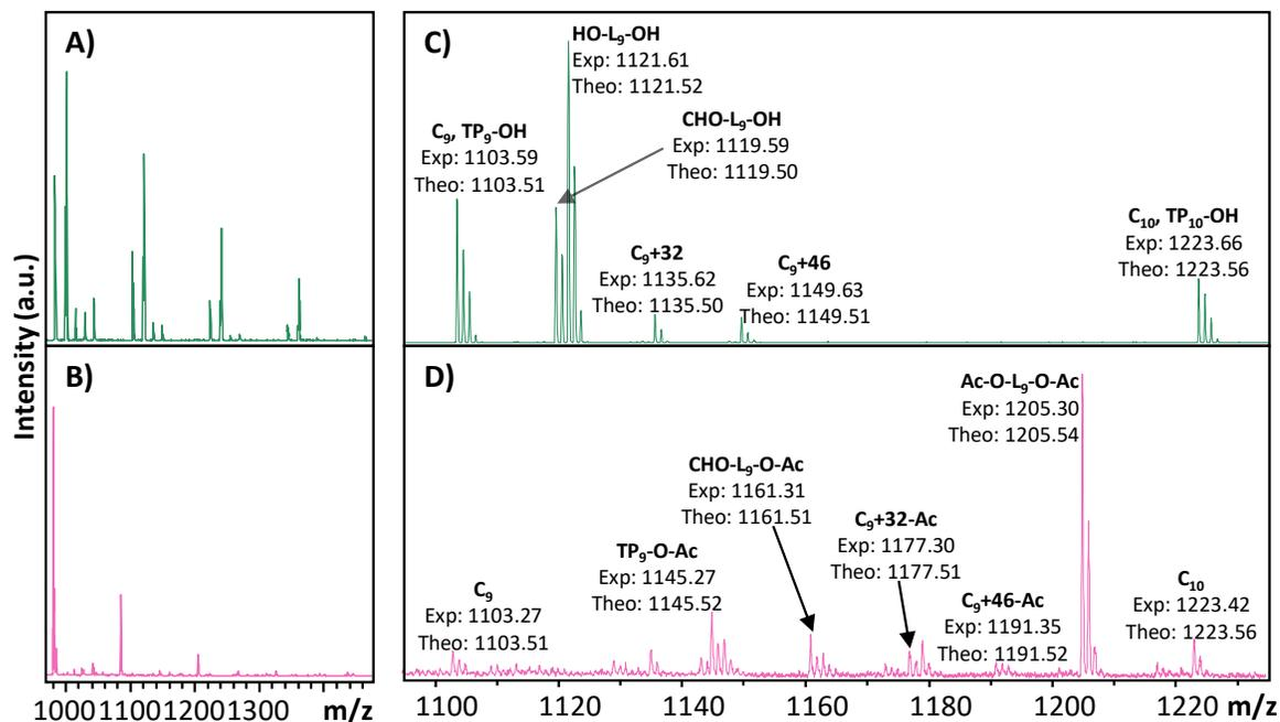
**Figure C7.** MALDI-ToF mass spectra of the low molecular poly(SO) fraction before (A,C) and after acetylation (B, D). Identification of signals is based on the end group functionalization. The spectra were acquired in positive reflector mode, and all signals represent the sodiated adducts.
