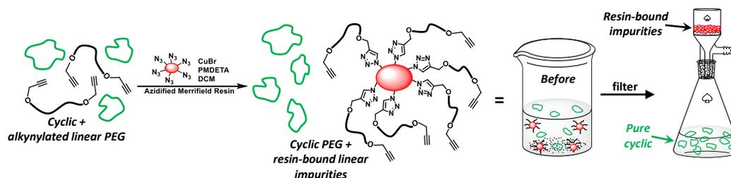
**Scheme 6.2.** “Click” scavenging purification protocol to remove unwanted linear impurities
