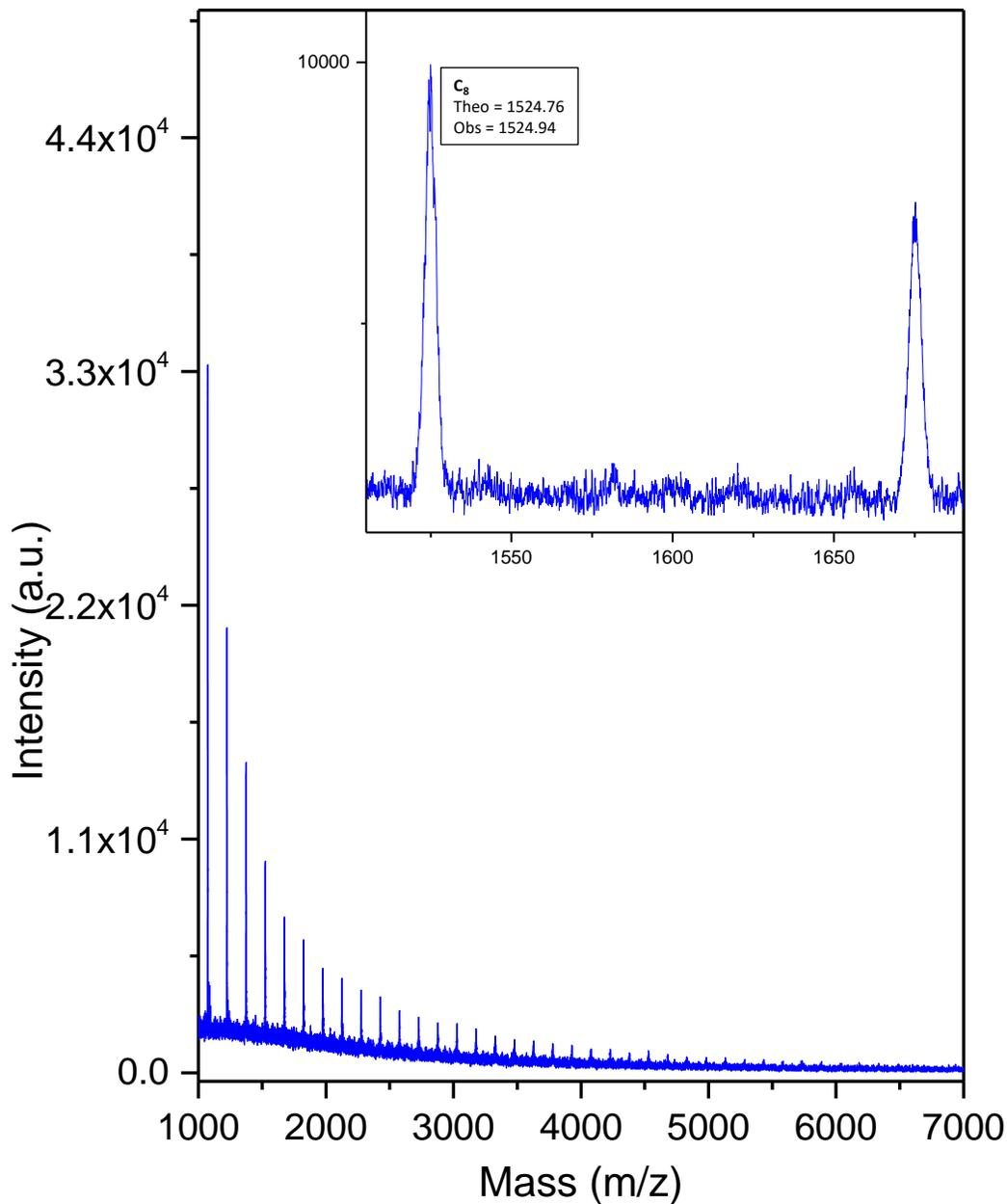
**Figure B12.** MALDI-ToF mass spectrum of “click-scavenged” poly(GPE)<sub>11K</sub> sample was taken in linear mode, and all labeled signals represent the sodiated adducts.
