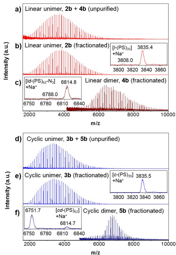
**Figure A4.** MALDI TOF mass spectra of a)  $l$ -PS<sub>2800</sub>, **2b** + **4b**, b)  $l$ -PS<sub>2800</sub>, **2b**, c)  $ld$ -PS<sub>2800</sub>, **4b**, and d)  $c$ -PS<sub>2800</sub>, **3b** + **5b**, e)  $c$ -PS<sub>2800</sub>, **3b**, f)  $cd$ -PS<sub>2800</sub>, **5b**. The theoretical  $m/z$  for the  $l$ - and  $c$ -PS 35-mer was 3835.5, the theoretical  $m/z$  for the metastable  $ld$ - and  $cd$ -PS 62-mer was 6814.8. 6751.7 peak in f) is cyclic unimer,  $c$ -PS 63-mer.
