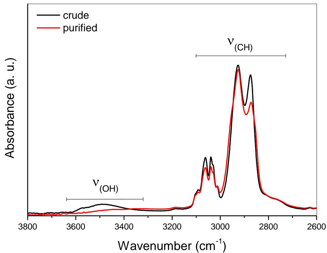
**Figure B14.** FTIR spectra of crude and purified cyclic poly(GPE)<sub>11K</sub>.
