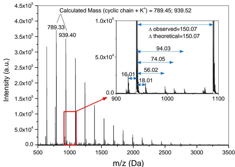
**Figure 3.1.** MALDI-TOF MS spectrum of cyclic poly(GPE)<sub>1K</sub> synthesized by ZREP. Inset: expanded m/z = 900-1120 region showing low intensity signals. Spectra were acquired using KTFA to provide a cation and DCTB as matrix.
