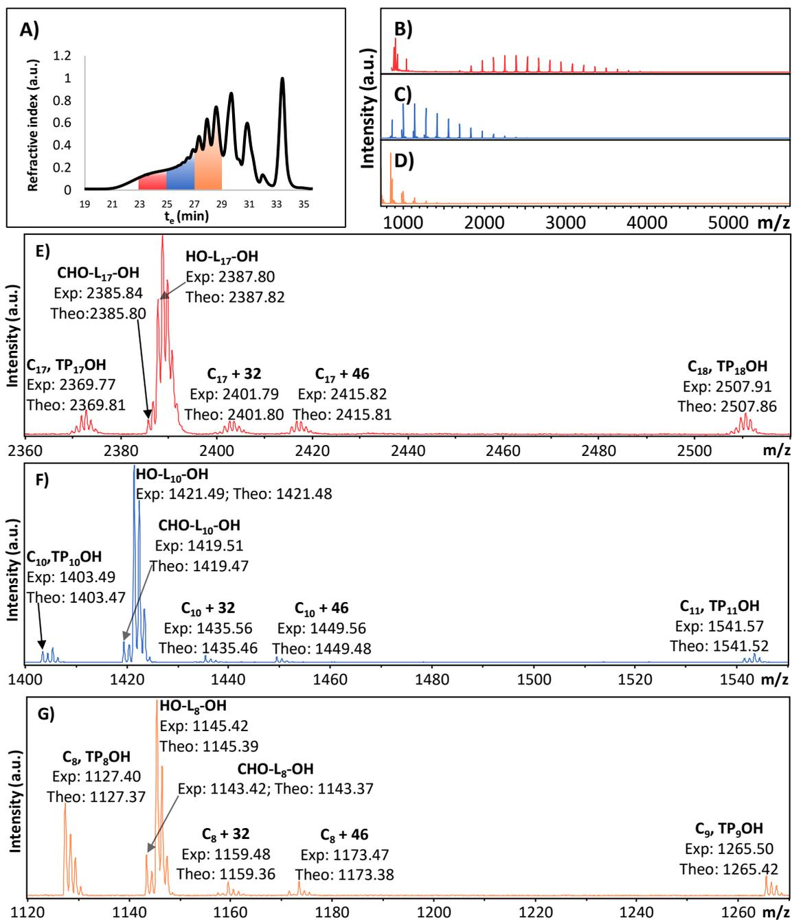
**Figure C10.** MALDI-ToF mass spectra of poly(F-SO) fractionated via SEC. The spectra were acquired in positive reflector mode, and all signals represent the sodiated adducts.
