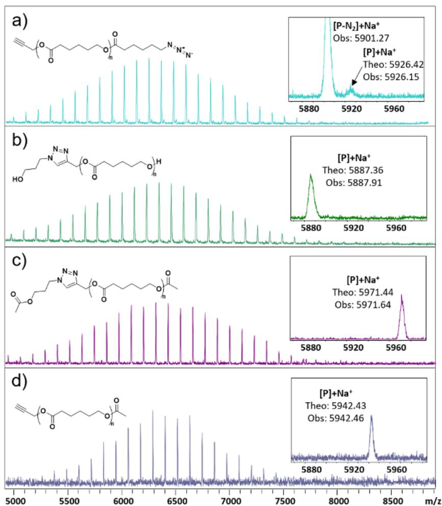
**Figure 5.5.** MALDI-TOF MS data illustrating the molecular weight distribution and purity of the four additional linear PCL controls: a)  $\alpha$ -propargyl- $\omega$ -azide-PCL; b) triazole-containing- $\alpha,\omega$ -dihydroxy-PCL; c) triazole-containing- $\alpha,\omega$ -diacetyl-PCL; d)  $\alpha$ -propargyl- $\omega$ -acetyl-PCL.
