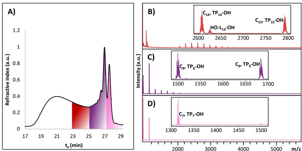
**Figure 4.2.** Poly(Cl-PGE) was fractionated by SEC (A), and the corresponding MALDI-ToF mass spectra of each SEC fraction is shown (B, C, and D). The spectra were acquired in reflector mode, and all signals represent the sodiated adducts.
