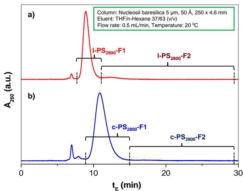
**Figure A1.** HPLC chromatograms during the separation and isolation of the unimer fraction 10 days after azidization and cyclization for a) *l*-PS<sub>2800</sub> and b) *c*-PS<sub>2800</sub>
