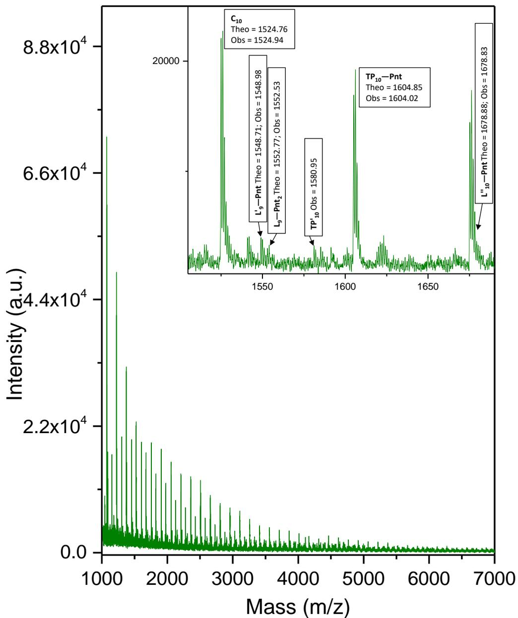
**Figure B11.** MALDI-ToF mass spectrum of pent-4-ynoated poly(GPE)<sub>11K</sub> sample was taken in linear mode, and all labeled signals represent the sodiated adducts.
