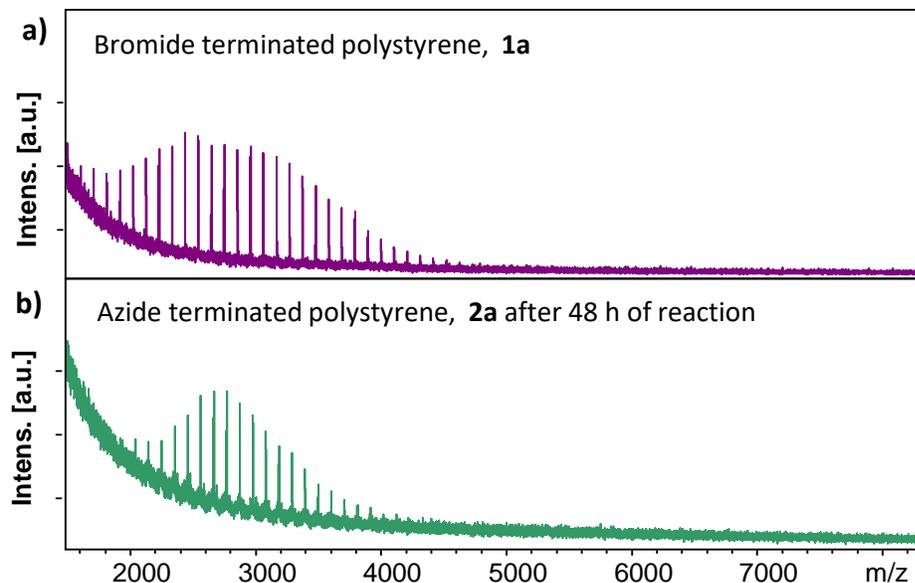
**Figure 2.5:** MALDI-TOF mass spectra of azidization reaction of **1a** to generate **2a** at a) 0h, and b) at 48 h exhibits no sign of “click” oligomerization.
