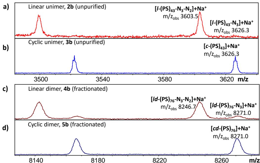
**Figure A5.** MALDI-TOF mass spectra in reflector mode of a) *l*-PS<sub>3700</sub>, b) *c*-PS<sub>3700</sub>, c) *ld*-PS<sub>3700</sub>, d) *cd*-PS<sub>3700</sub> confirming the loss of the predominant metastable azide signal upon CuAAC cyclization to form the triazole linkage in the cyclic products.
