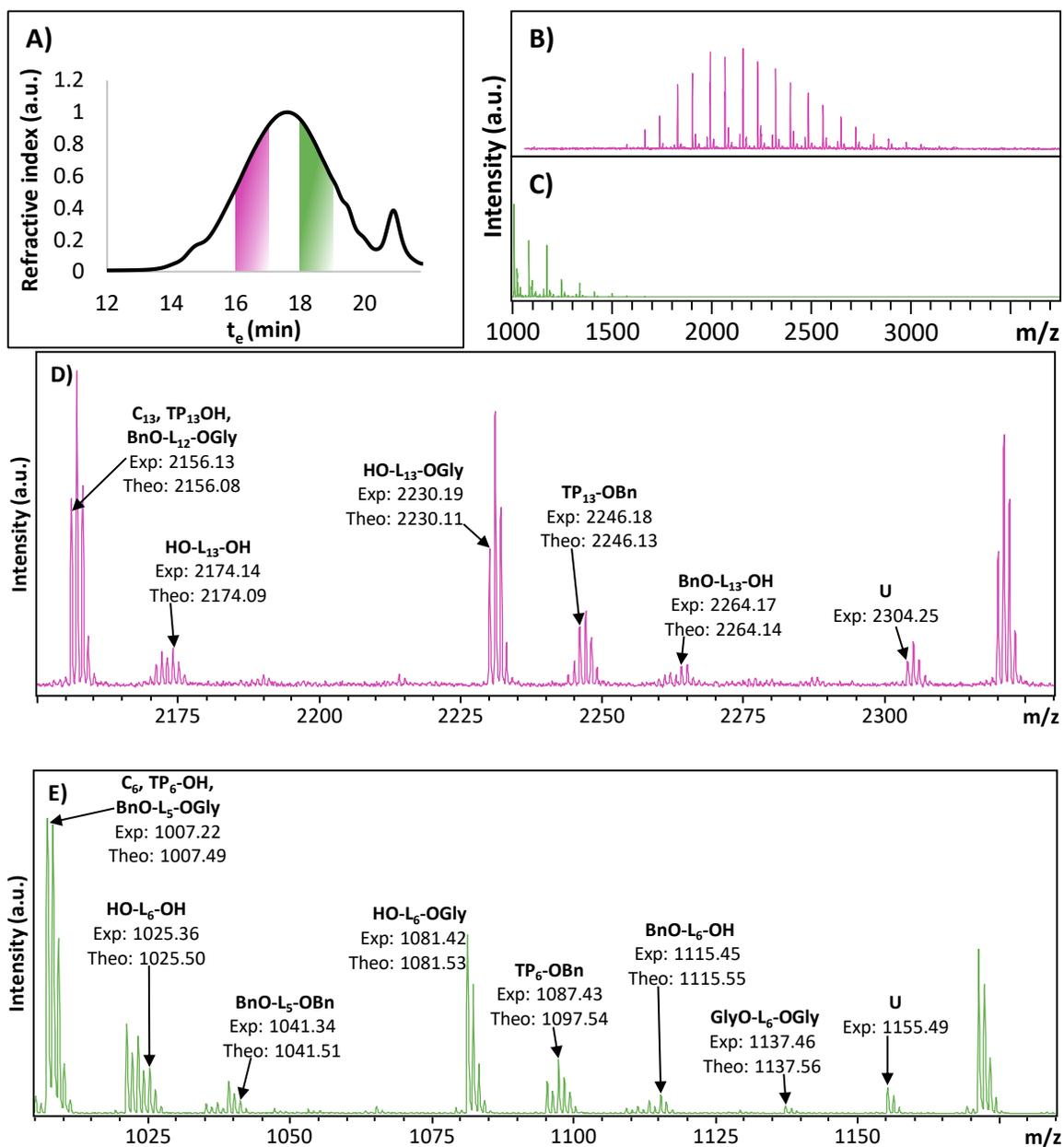
**Figure C3.** Poly(BGE) was fractionated by SEC (A), and the corresponding MALDI-ToF mass spectra of each SEC fraction is shown with full spectra (B and C) and corresponding insets (D and E).
