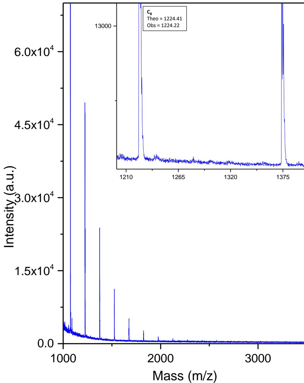
**Figure B9.** MALDI-ToF mass spectrum of “click-scavenged” poly(GPE)<sub>11K</sub> sample was taken in positive reflector mode, and all labeled signals represent the sodiated adducts.
