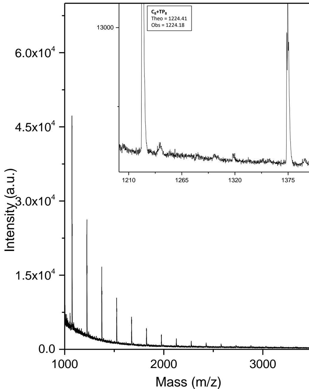
**Figure B7.** MALDI-ToF mass spectrum of crude poly(GPE)<sub>11K</sub> sample was taken in positive reflector mode, and all labeled signals represent the sodiated adducts.
