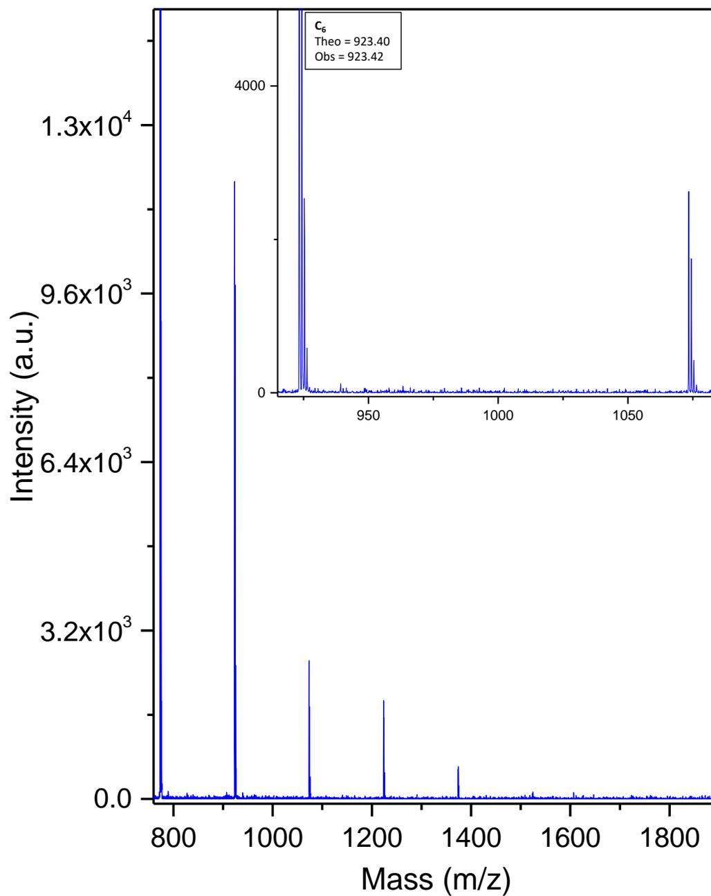
**Figure B3.** MALDI-ToF mass spectrum of “click-scavenged” poly(GPE)<sub>1K</sub> sample was taken in positive reflector mode, and all labeled signals represent the sodiated adducts.
