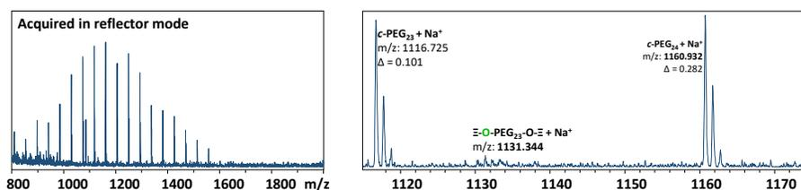
**Figure 6.3.** MALDI-TOF MS data of the cyclic PEG
