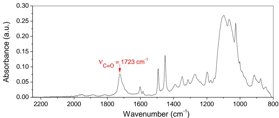
**Figure C8.** FTIR data of poly(SO) indicating the formation of carbonyl groups in the SO polymer series resulting from the initiation of polymerization with phenylacetaldehyde.
