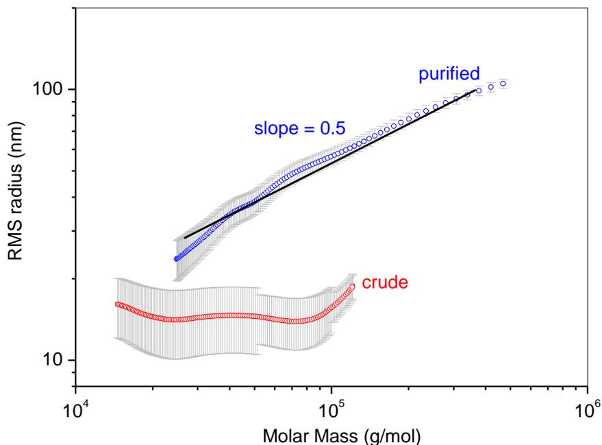
**Figure 3.8.** Conformation plot for crude and purified poly(GPE)<sub>11K</sub>.
