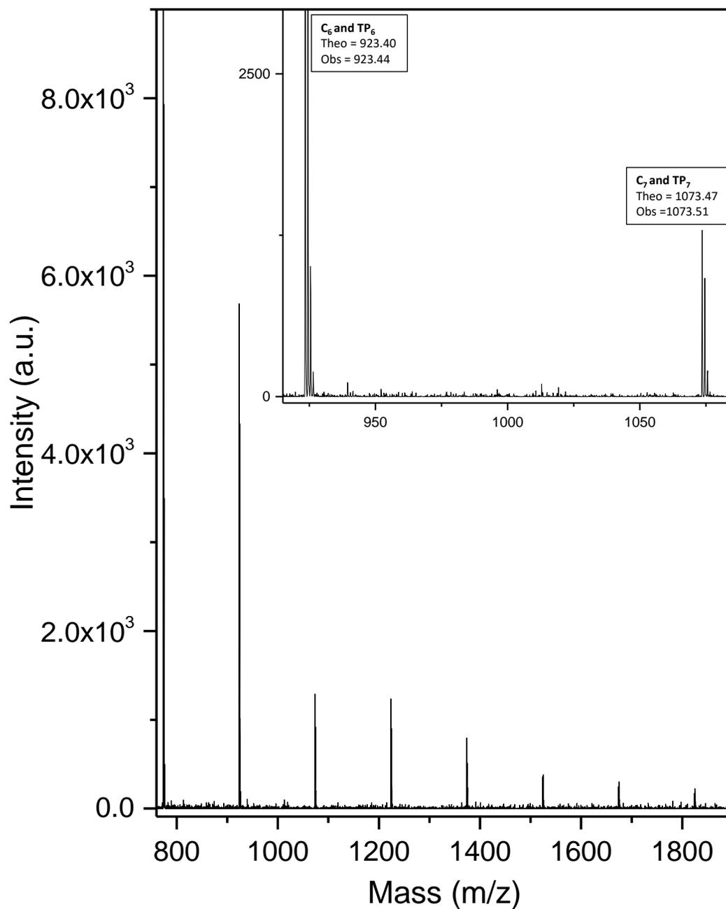
**Figure B1.** MALDI-ToF mass spectrum of crude poly(GPE)<sub>1K</sub> sample was taken in positive reflector mode, and all labeled signals represent the sodiated adducts.
