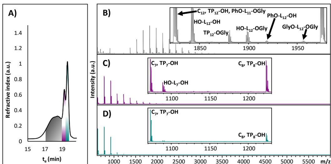
**Figure 4.1.** Poly(PGE) was fractionated by SEC (A), and the corresponding MALDI-ToF mass spectra of each SEC fraction is shown (B, C, and D). Identification of signals is based on the end group functionalization performed in a previous study.<sup>18</sup> The spectra were acquired in reflector mode, and all signals represent the sodiated adducts.
