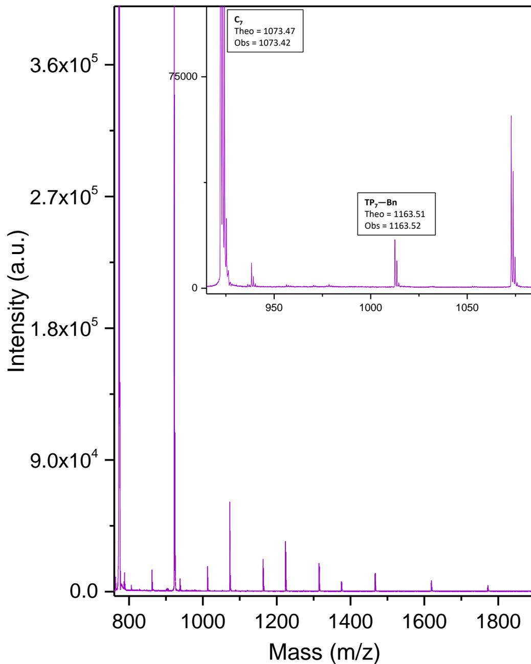
**Figure B5.** MALDI-ToF mass spectrum of benzylated poly(GPE)<sub>1K</sub> sample was taken in positive reflector mode, and all labeled signals represent the sodiated adducts.
