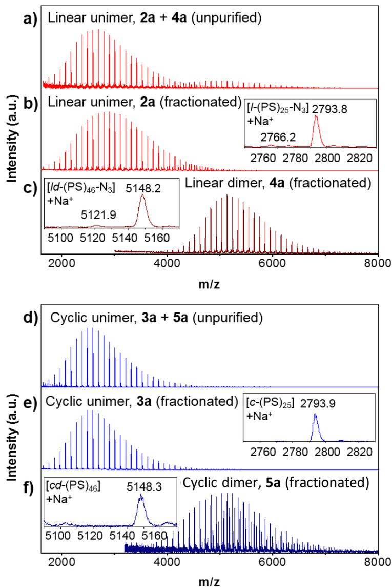
**Figure 2.2.** MALDI TOF mass spectra of samples in linear mode before and after fractionation: a) unpurified *l*-PS<sub>2800</sub>, **2a** + **4a**, b) purified *l*-PS<sub>2800</sub>, **2a**, c) purified *ld*-PS<sub>2800</sub>, **4a**, and d) unpurified *c*-PS<sub>2800</sub>, **3a** + **5a**, e) purified *c*-PS<sub>2800</sub>, **3a**, and f) purified *cd*-PS<sub>2800</sub>, **5a**
