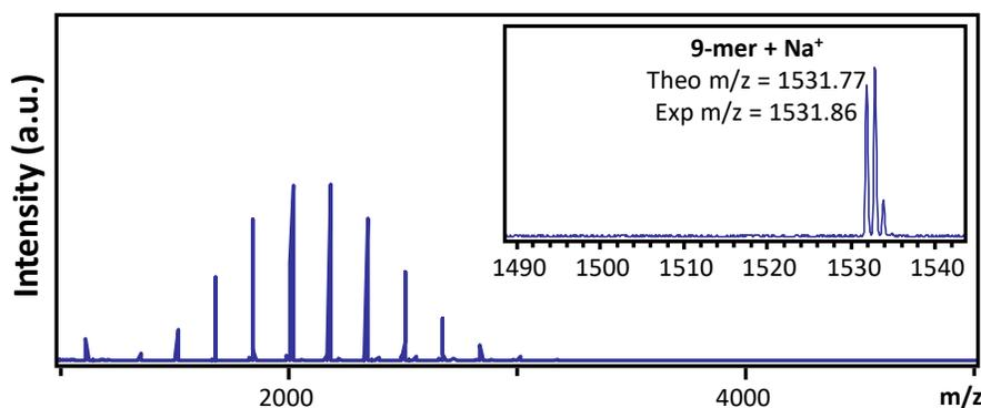
**Figure 6.5.** MALDI-TOF of methanol initiated poly(glycidyl 2-methylphenyl ether)
