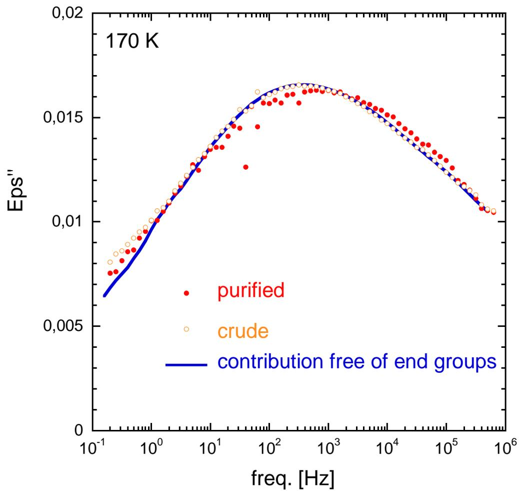
**Figure B15.** Frequency dependence of the  $\epsilon''$  for the  $\beta$ -relaxation of crude and purified poly(GPE)<sub>11K</sub> sample at 170K. Solid line shows the contribution to local dynamics of side groups (end groups are excluded), as previously obtained from linear poly(GPE) samples in reference S<sup>1</sup>.
