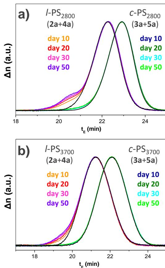
**Figure 2.3:** SEC chromatograms of  $l$ -PS and  $c$ -PS at days 10, 20, 30, and 50, (post-synthesis). Black traces are for the HPLC fractionated unimers.
