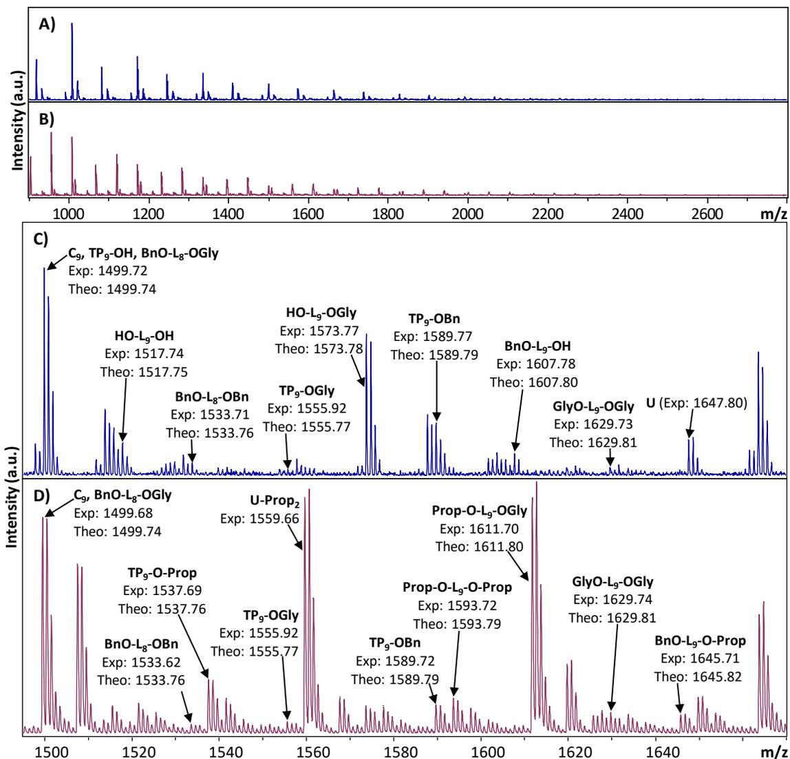
**Figure C4.** MALDI-ToF mass spectra of crude poly(BGE) (A,C) and propargylated poly(BGE) (B, D). Identification of signals is based on the end group functionalization. The spectra were acquired in positive reflector mode, and all signals represent the sodiated adducts.
