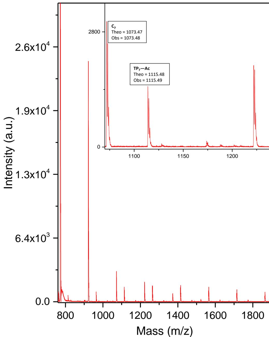
**Figure B4.** MALDI-ToF mass spectrum of acetylated poly(GPE)<sub>1K</sub> sample was taken in positive reflector mode, and all labeled signals represent the sodiated adducts.
