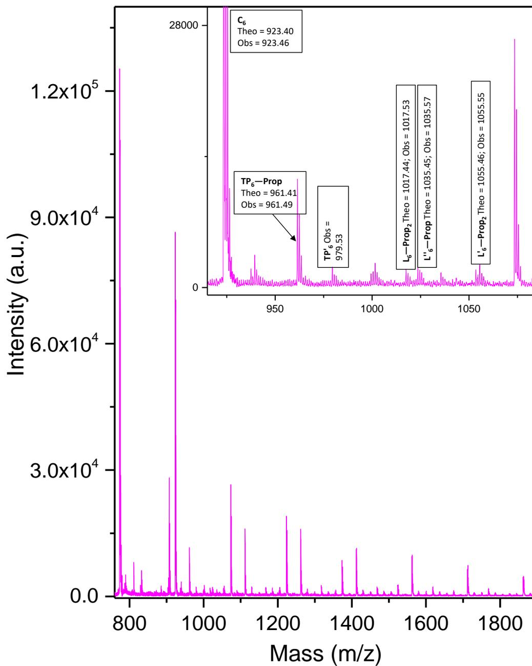
**Figure B2.** MALDI-ToF mass spectrum of propargylated poly(GPE)<sub>1K</sub> sample was taken in positive reflector mode, and all labeled signals represent the sodiated adducts.
