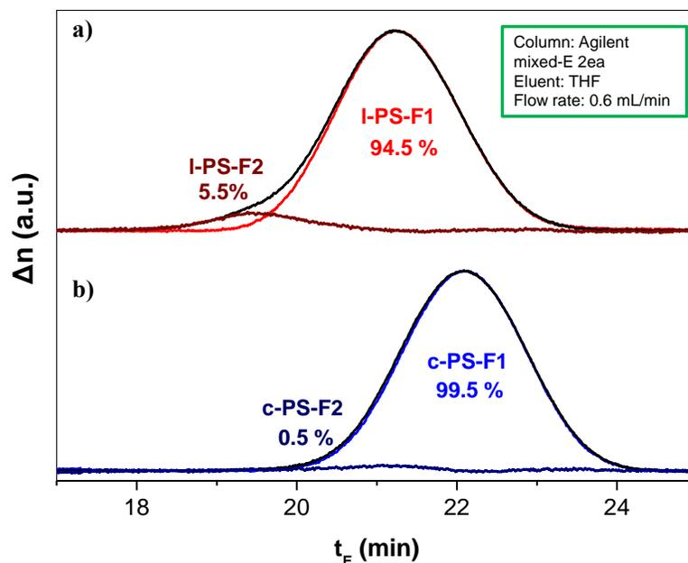
**Figure A7.** Representative SEC chromatograms of HPLC fractions 30 days after azidization and cyclization for a) *l*-PS<sub>3700</sub> and b) *c*-PS<sub>3700</sub>. Fraction 1 corresponds to the isolated unimer fraction, while fraction 2 corresponds to the dimer fraction.
