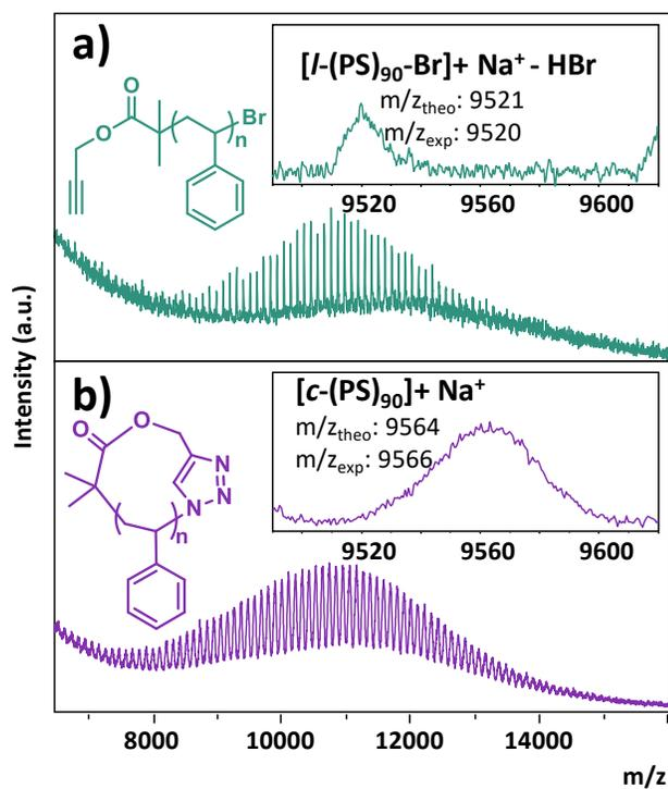
**Figure 2.7.** MALDI-TOF MS spectra of *l*- and *c*-PS<sub>10k</sub> with expanded spectra from  $m/z = 9490$  to  $9620$  confirm quantitative end group and architectural transformation.
