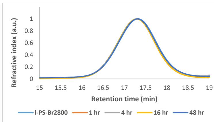
**Figure 2.4:** SEC chromatograms of azidization reaction of **1a** to generate **2a** at 1h, 4 h 16 h and 48h show no sign of click oligomerization.
