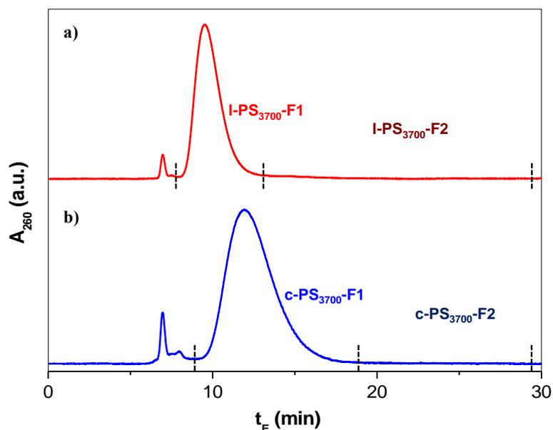
**Figure A2.** HPLC chromatograms during the separation and isolation of the unimer fraction 10 days after azidization and cyclization for a) *l*-PS<sub>3700</sub> and b) *c*-PS<sub>3700</sub>
