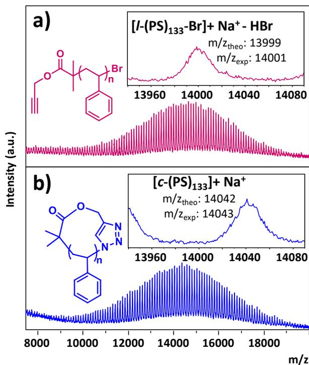
**Figure 2.8.** MALDI-TOF MS spectra of *l*- and *c*-PS<sub>14k</sub> with expanded spectra from  $m/z = 13940$  to  $14090$  confirm quantitative end group and architectural transformation.
