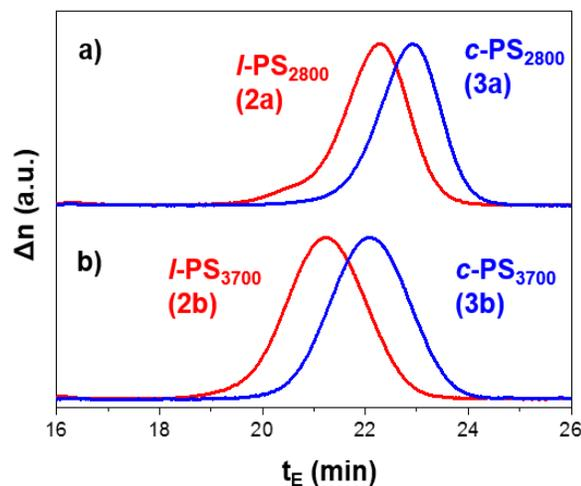
**Figure 2.1.** SEC chromatograms of a) *l*-PS<sub>2800</sub> (**2a**) and *c*-PS<sub>2800</sub> (**3a**) 10 days after click cyclization, b) *l*-PS<sub>3700</sub> (**2b**) and *c*-PS<sub>3700</sub> (**3b**) 10 days after click cyclization.
