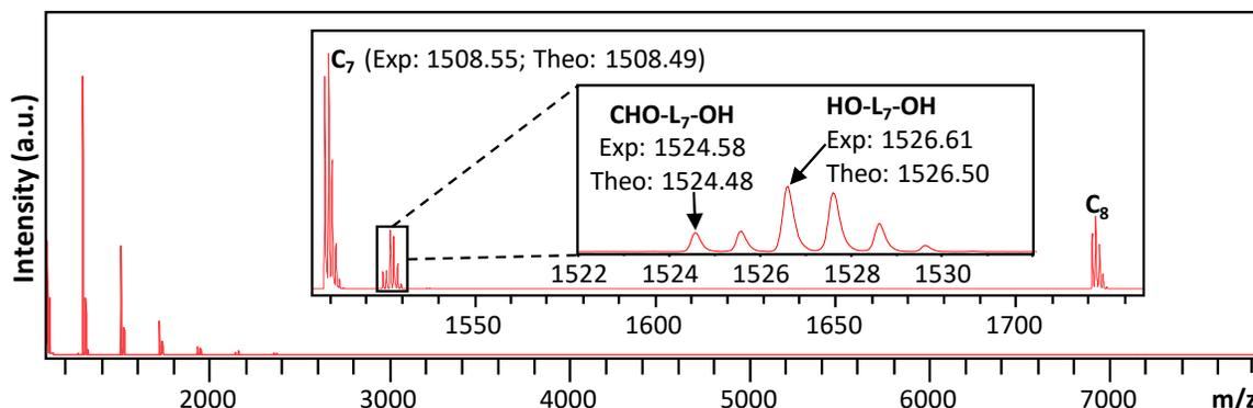
**Figure C5.** MALDI-ToF mass spectra of the mid-molecular weight fraction of poly(ETD) collected via SEC. Identification of signals is based on the end group functionalization (Figure C5). The expanded spectra illustrates that there are two overlapping signals, CHO-L7-OH and HO-L7-OH. The spectrum was acquired in positive reflector mode, and all signals represent the sodiated adducts.
