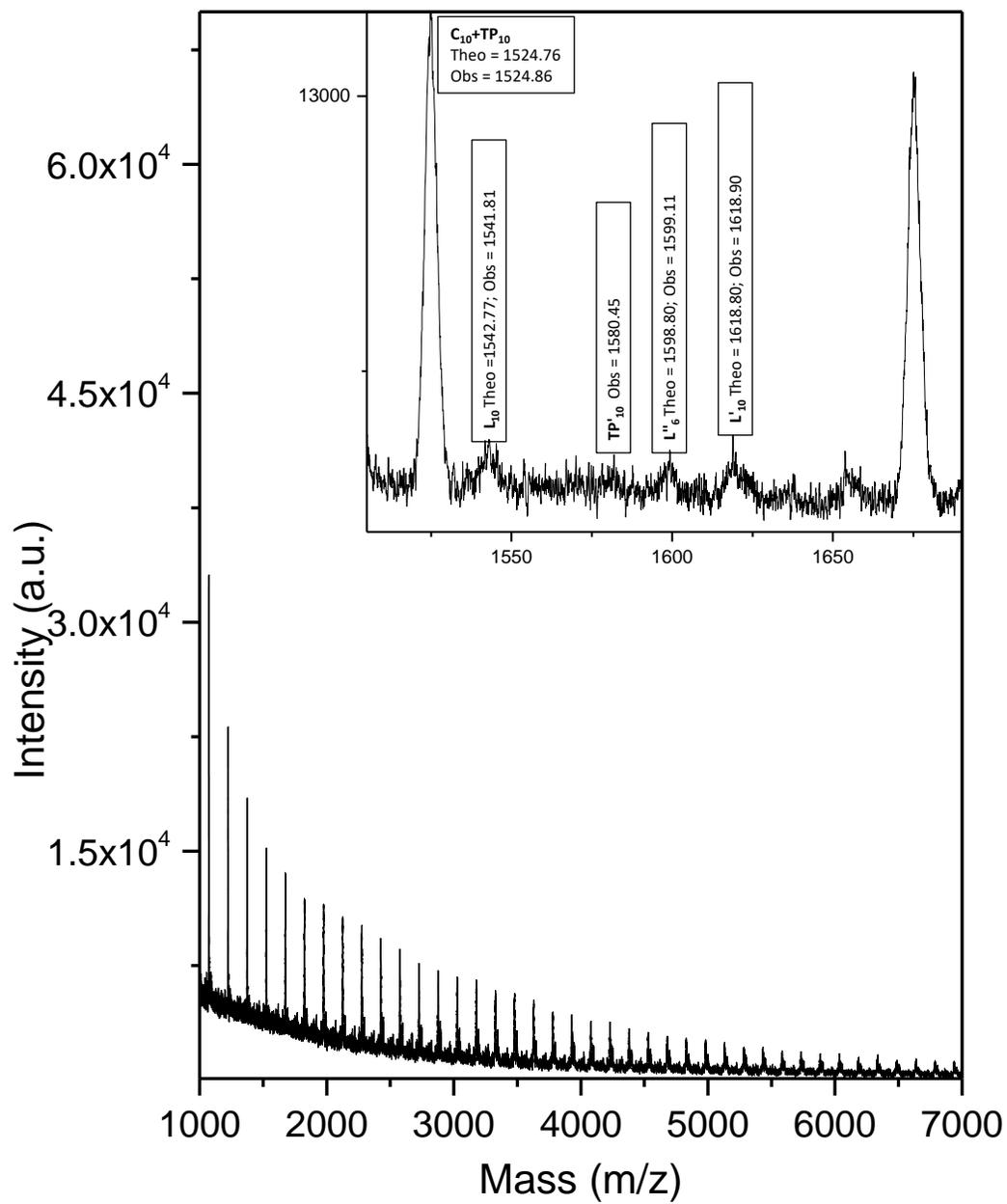
**Figure B10.** MALDI-ToF mass spectrum of crude poly(GPE)<sub>11K</sub> sample was taken in linear mode, and all labeled signals represent the sodiated adducts.
