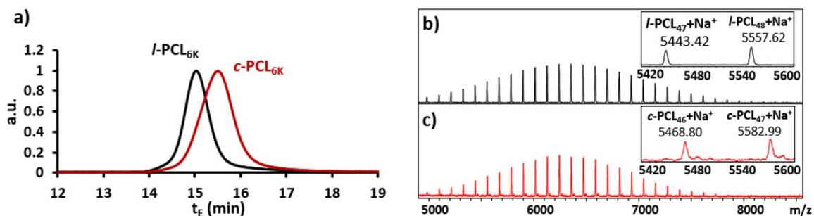
**Figure 5.2.** Molecular weight characterization data for *l*-PCL<sub>6k</sub> and *c*-PCL<sub>6k</sub>. a) GPC chromatograms illustrate the longer elution time for the *c*-PCL<sub>6k</sub> due to its decreased hydrodynamic radius. b-c) MALDI-TOF MS spectra of *l*-PCL<sub>6k</sub> and *c*-PCL<sub>6k</sub> indicate exceptional uniformity in both species with respect to end group functionalities and architectural transformations.
