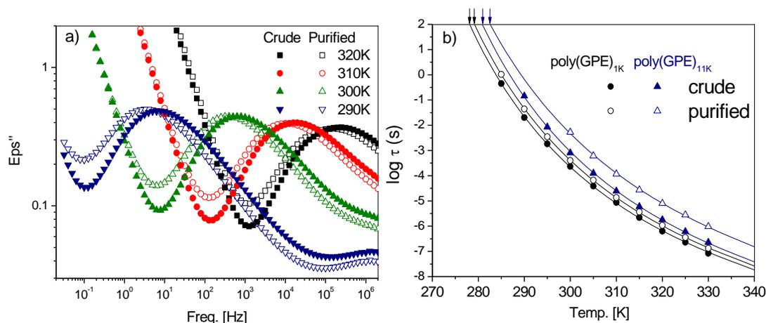
**Figure 3.10.** a) Dielectric relaxation for crude and purified poly(GPE)<sub>1K</sub> at temperatures above glass transition. b) Temperature dependence of the  $\alpha$ -relaxation times for crude and purified cyclic poly(GPE) samples. Arrows indicate the dynamic (dielectric) glass transition temperatures,  $T_g^{BDS}$ .
