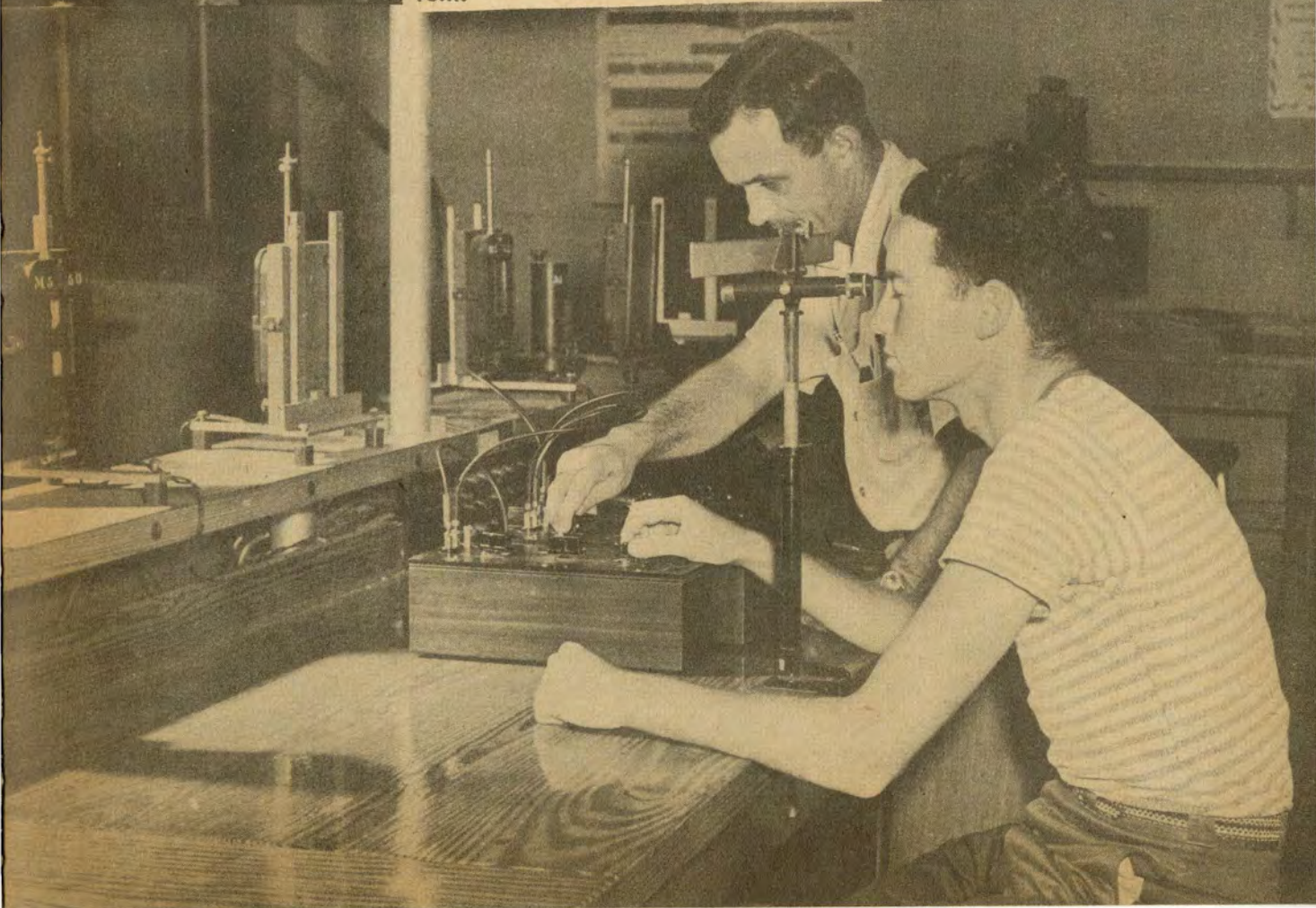
It looks like a giant wagon wheel, but actually is part of a steam engine. Below, a galvanometer and a small telescope are used to measure electric current.
